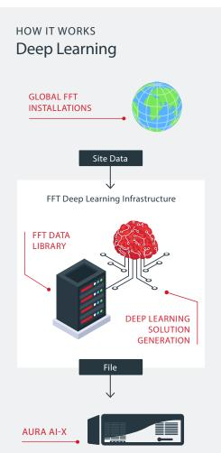
Data from FFT's extensive global system installations is used to train effective Deep Learning models deployed to an Aura Ai-X system via encrypted file transfer. The Deep Learning engine in Aura Ai-X uses this model to perform real-time detection and classification of events monitored on the fiber sensor.
